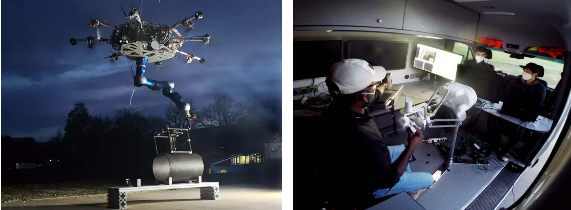
Figure 1. Left: the cable-Suspended Aerial Manipulator, dubbed SAM (Sarkisov et al., 2019) during field experiments. Right: a ground station where an operator remotely controls the robotic arm through a haptic interface. In real world applications of bilateral teleoperation, the operator is often remotely located without visual contact to the robot.
