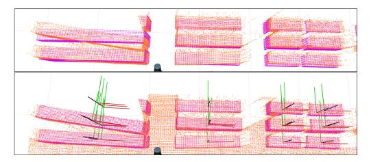
**Figure 11.** Precise alignment of individual bricks. Laser measurements are colored orange, model points are shown in purple. Top: Initial solution found by the rough ICP stage. Bottom: Resulting brick poses. The scan was captured during a competition run.
