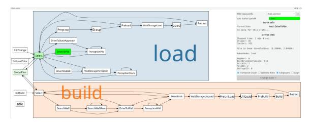
**Figure 5.** Graphical user interface showing all states of the FSM developed for Challenge 2. User defined information are shown in the status bar on the right. The active state is highlighted in green. The operator can perform state transitions manually using this GUI.
