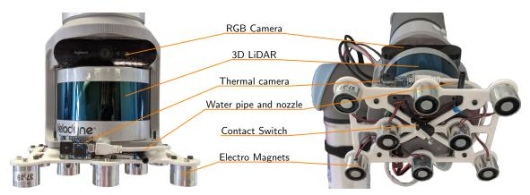
Figure 4. Front (left) and bottom view (right) of our end-effector which incorporates multiple vision sensors, magnets for grasping purposes, a contact switch and a nozzle for water dispensation.
