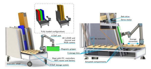
**Figure 3.** Left: UGV hardware design. Top: The storage system is capable of holding either 10 orange bricks (left) or all remaining bricks (20 red, 10 green, 5 blue) (right). Right: Actuated storage system.
