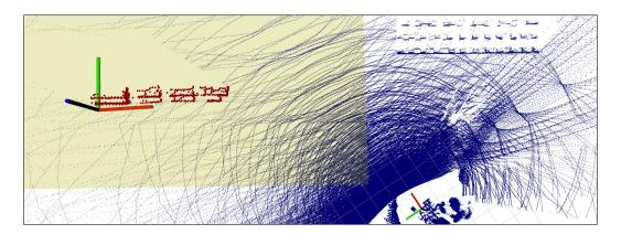
**Figure 9.** Pile detection from LiDAR points (blue). The robot is located at the small coordinate system (bottom). The search area can be restricted using geofencing (yellow rectangle). Detected points are visualized in red and the estimated pile pose is shown. The scan was captured inside the competition arena during a test run.
