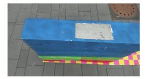
**Figure 16.** Experiment: Two example results building a predefined wall structure fully autonomously. Tiny differences in the brick alignment can be seen at the green bricks.
