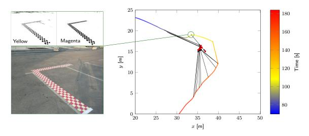
**Figure 13.** Marker detection during practice run. The robot was teleoperated through the arena, driving past the marker. Bob's trajectory is shown colored by time. Each detection is shown as a red square, with an arrow from Bob's position at detection time. The images on the left show an example scene captured at the green circle including the yellow and magenta color mask output.
