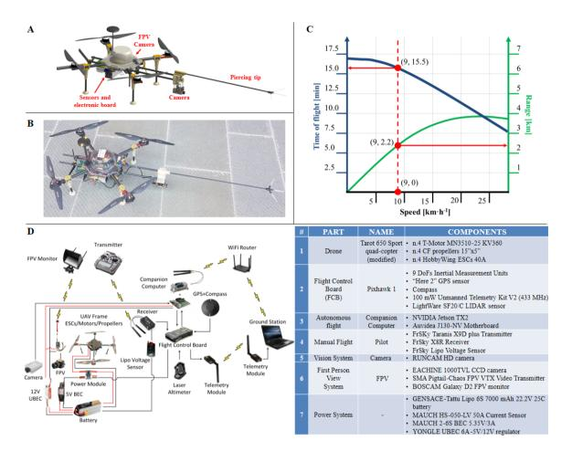
**Figure 2.** Hardware architecture of the drone. Panels A, B. 3D CAD model of the drone and actual realization of the platform. Panel C. Drone performance estimated by xcopterCALC Software (Müller, 2020). Panel D. Deployment of the hardware components and their functional connections.
