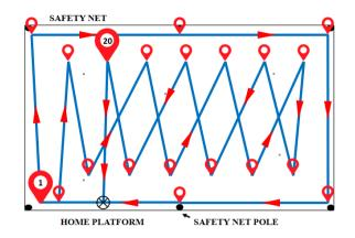
Figure 9. Waypoints: pre-set GPS points that define the searching trajectory of the drone.
