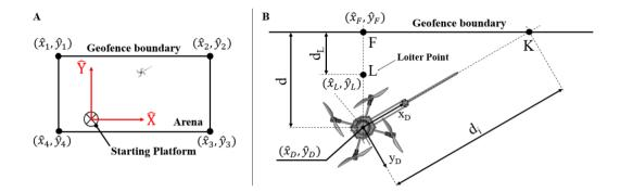
**Figure 12.** The *Geo-fence State*.Panel A: definition of the Geofence boundaries and identification of the reference frame centered on the starting platform. Panel B: Geometrical analysis for the *Geo-fence State*. Note. Table 1 reports the description of the parameters employed in the Figure.
