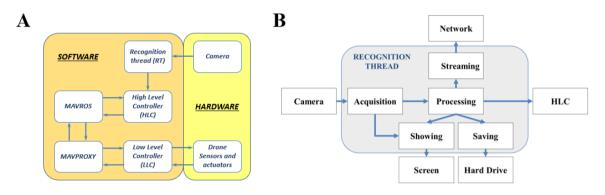
**Figure 4.** Multi-thread software structure. Panel A. Software architecture and interface with the hardware components. The HLC manages the robotic platform with a state machine that exploits the information given by drone sensors and actuators through the LLC and the MAVROS/MAVPROXY modules and data from the recognition thread that elaborates the images acquired by the online camera. Panel B: Multi-thread structure of the vision system.
