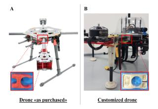
**Figure 3.** Structural modifications to enhance a mechanical stability. Panel A. Tarot 650 Sport quad-copter as purchased (picture from the web). The detail shows the V-shape connection between the main frame and the arm. Panel B. Drone customized by substituting the joints with an aluminum clamp and by providing a new fixed landing support placed at arm extremity.
