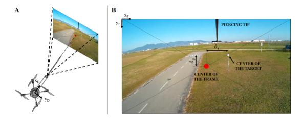
**Figure 7.** Qualitative depiction of the drone capturing a frame in the surrounding environment (Panel A). Panel B shows the main features ( $\delta_x$  and  $\delta_y$ ) extracted from the frame.
