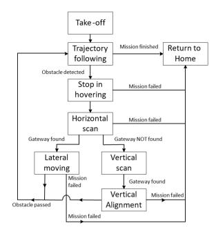
Figure 16. State Machine for Obstacle Avoidance tested with I-SIMC.
