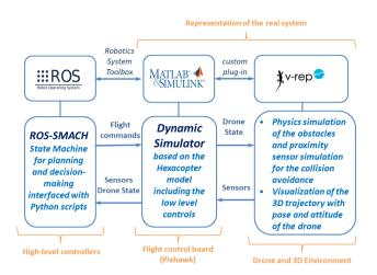
Figure 14. I-SIMC Architecture with which we simulated the aerial platform.
