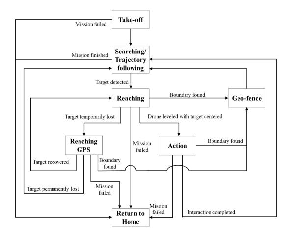
Figure 8. Main State Machine of the High level controller (HLC).
