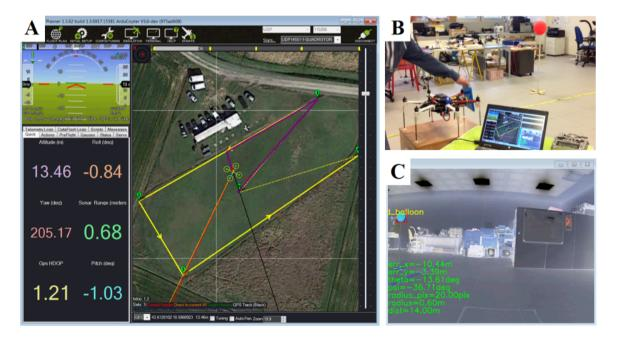
**Figure 13.** Pictures taken during a simulation test at our laboratory in Livorno (Italy). Panel A. Mission Planner graphics to visualize the simulated trajectory and sensor data from SITL. Panel B. Laboratory trials to frame a target with the on-board camera. Panel C. Showing thread graphics from the RT with the processed frames.
