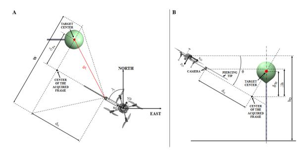
**Figure 11.** Alignment with the target. Panel A. View from a plane passing through the camera and angled by  $\vartheta$  (pitch angle) with respect to the horizontal line. Panel B. Vertical alignment with compensation of the pitch angle. Note. Table 1 reports the description of the parameters employed in the Figure.
