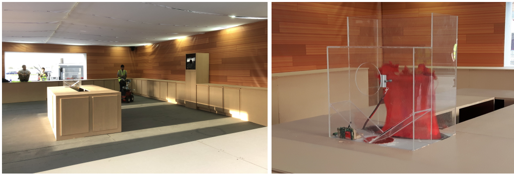
Figure 3. Left: Indoor area of the Challenge 3 arena. Right: Simulated indoor fire containing a heated plate and a moving red fabric, and a glass container to collect and measure the water deposited by the robots.
